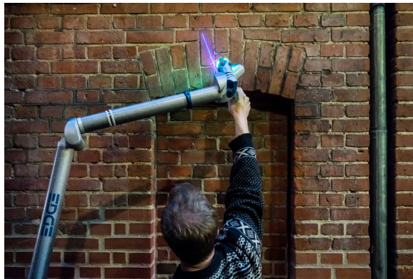
High-resolution detail scanning using the handheld FARO Edge Arm. This type of scanning is a manual process that requires direct engagement with the material and continuous evaluation of the scanning result.
