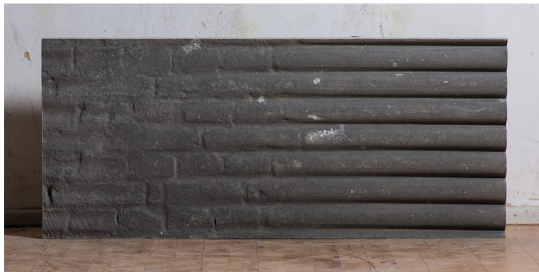
Brick Transition. The concrete casting of merged computer-made geometry and texture from the digitisation of reality.
