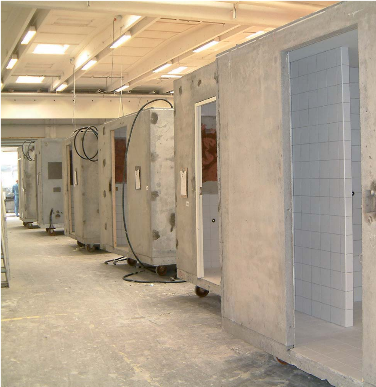
Prefabricated bathroom pods. EJ Badekabiner. Photo: CINARK
