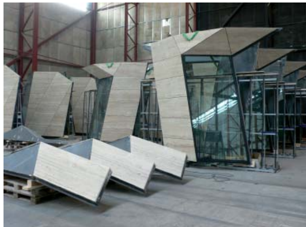
Prefabricated facade elements for the Horten Headquarters. 3xN photo: 3xN
