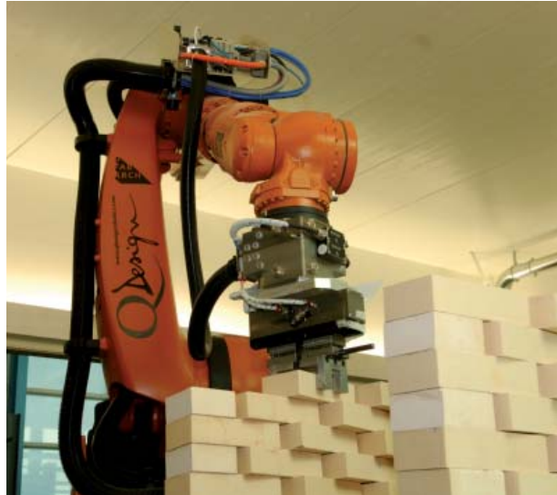
Wall building robot. Gramazio & Kohler ETH Zurich
