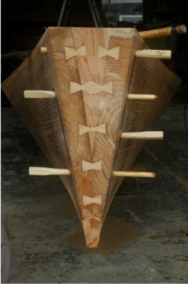
A view of the bow of the Sabani (fishing boat from Tohoku area) showing the huundu fastenings, along with cedar tunnels used to fasten the bow transome. Photograph by Douglas Brooks.
