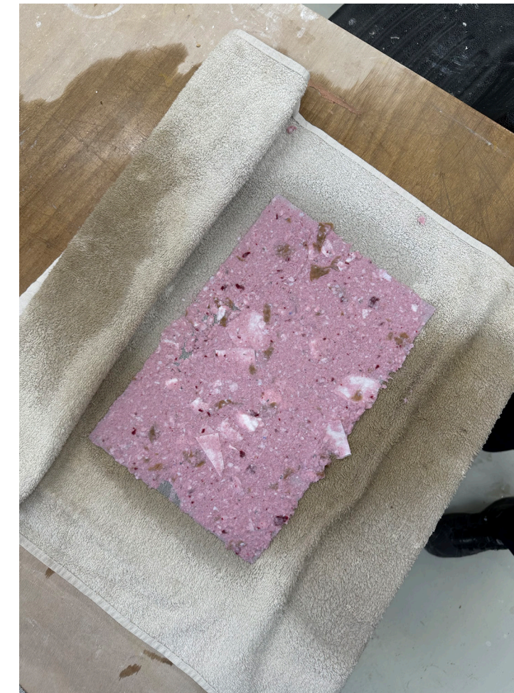
extract a layer of pulp on a flat drain/net and place on a towel, drain as much water as possible out and let dry
