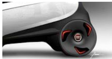
Letting the body of the car go over the wheels gives more room for interior space.
