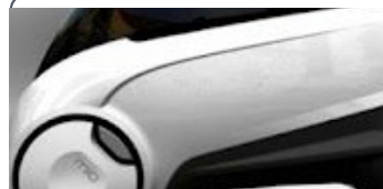
Letting the body of the car go over the wheels gives more room for interior space.
