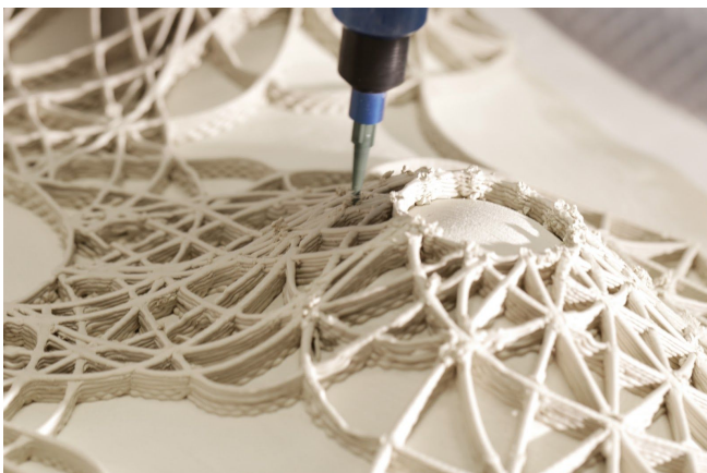
Fig. 3: Robotic 3d printing with porcelain in the Filigree Robotic project.
