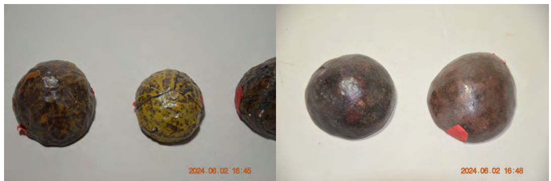
Figure 13 - test for blåler earthenware slip applied and high fired
