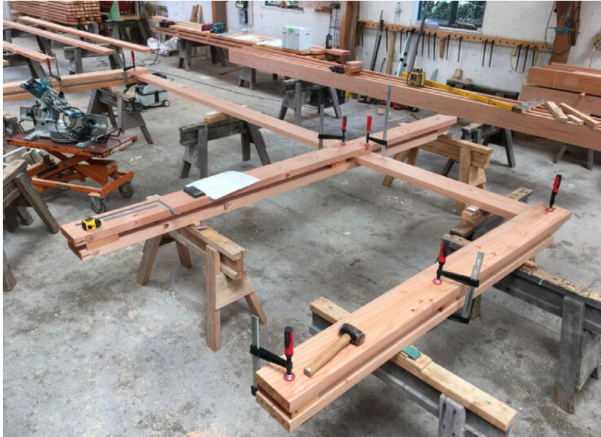
Fig. 35. Assembly of The Alice Hawthorn Inn, Yorkshire, The Timber Workshop
