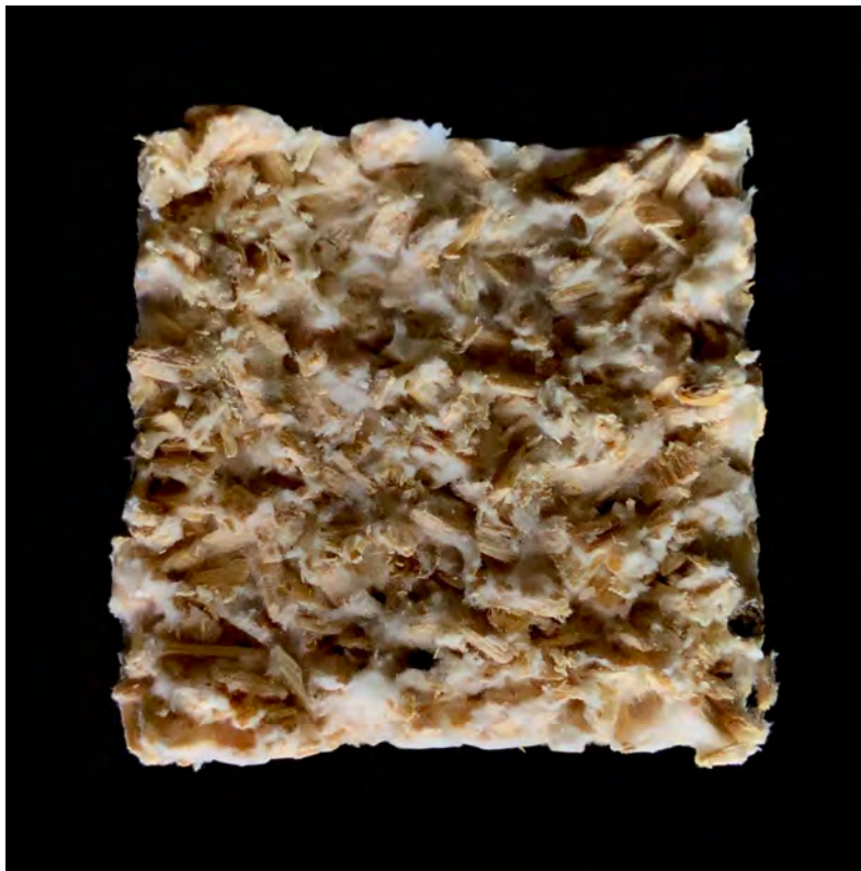
Figure 3.43: Section of a mycoboscutus cultivated on medium sized particles.
