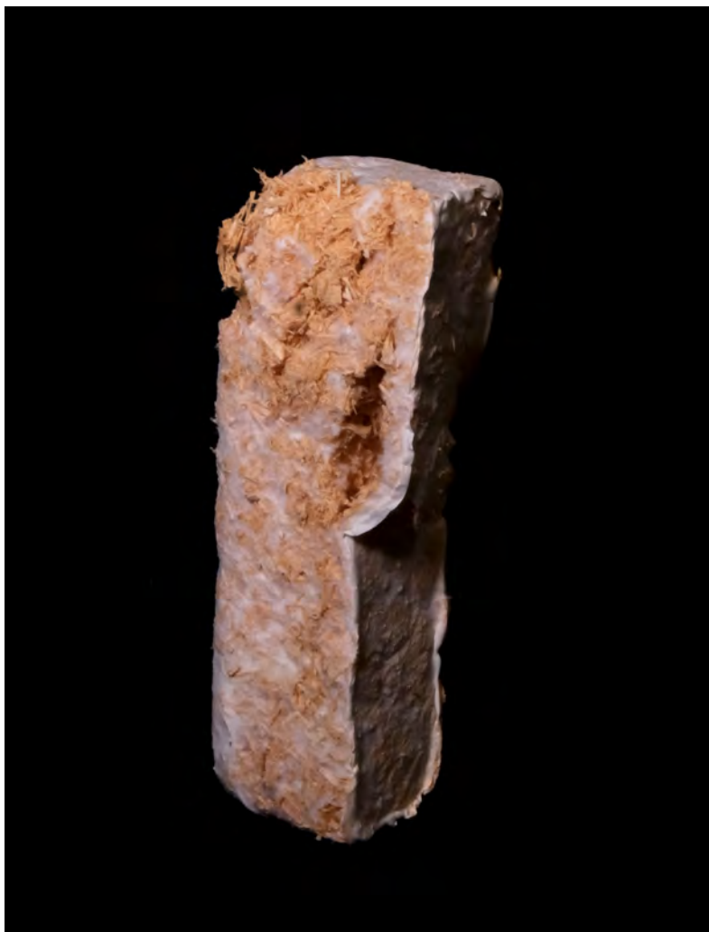
Figure 3.41: One specimen of G. lucidum colonised pine wood used for compressive characterisation, after having been tested.
