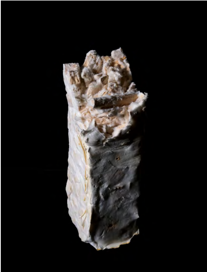
Figure 3.30: Rattan embedding specimen used for compressive characterisation, after having been tested.
