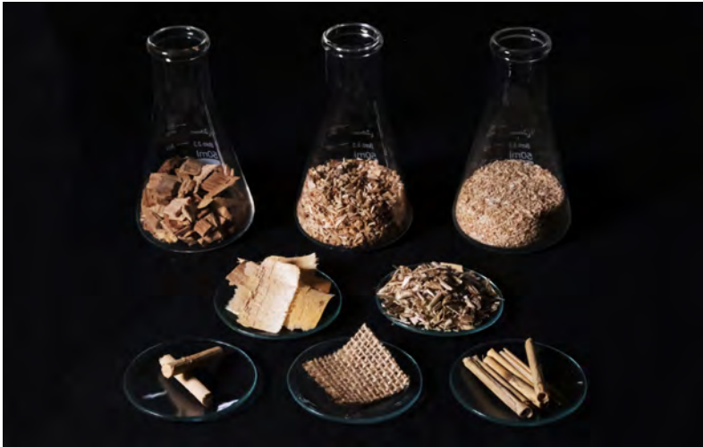
Figure 3.2O: Materials of the experimental studies (left to right, top to bottom): beech large (BL), beech medium (BM), beech small (BS), birch shavings (not used), hemp shives (not used), rattan fibres, hessian, and common reed fibres (2021).
