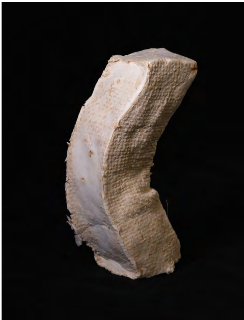
Figure 3.31: Hessian jacketed specimen used for compressive characterisation, after having been tested.
