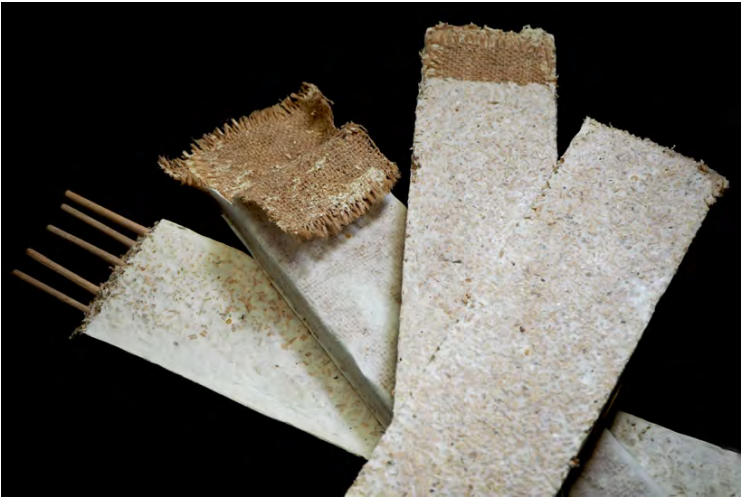
Figure 3. Fibre placement strategies in tested specimens (left to right): rattan fibres (BM_R), hessian jacketing (BM_H), inner hessian (BM_I), control (BM).
