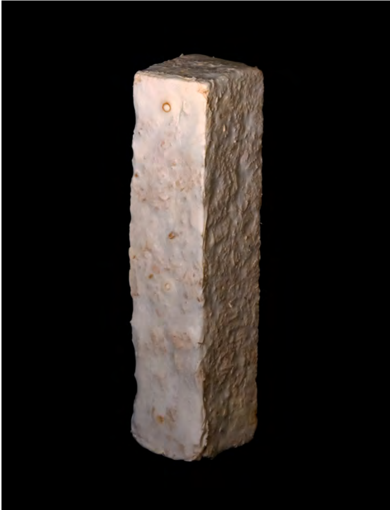
Figure 3.27: One dried specimen from the compression series.
