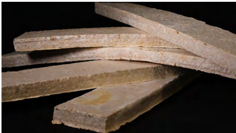
Figure 3.36: Standard cultivated specimens used for flexural characterisation, after having been tested.
