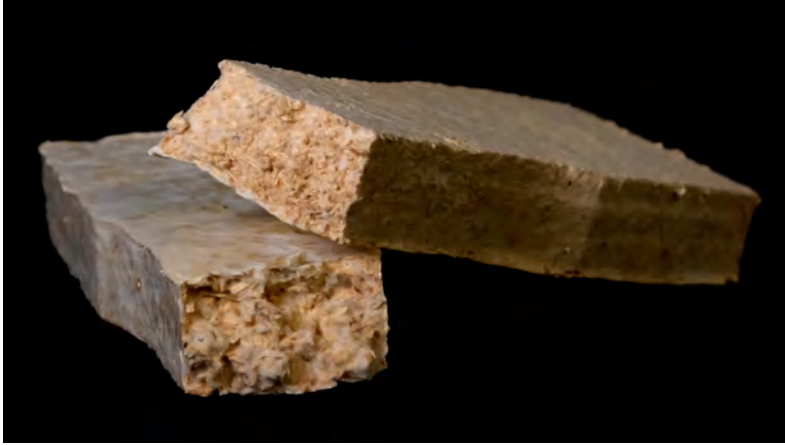
Figure 3.33: Two of the specimens tested for tensile characterisation (BM and BS-based); notice the arrangement of particles and mycelium in the section.
