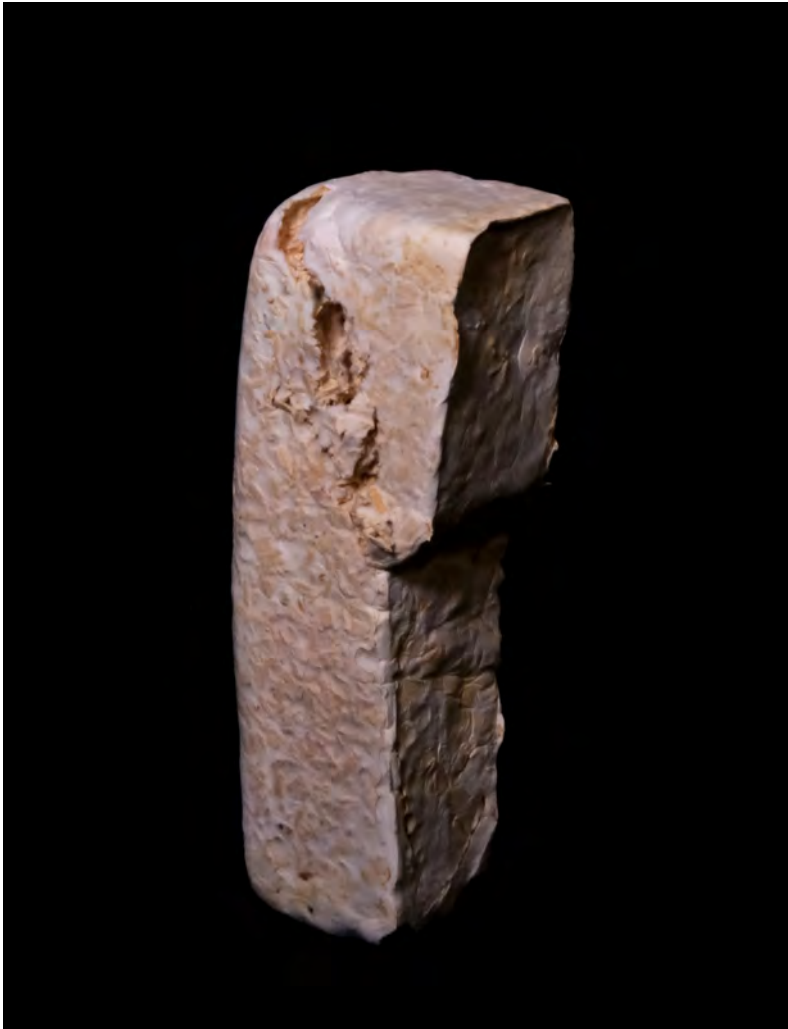
Figure 3.42: One specimen of G. resinaceum colonised beech wood used for compressive characterisation, after having been tested.
