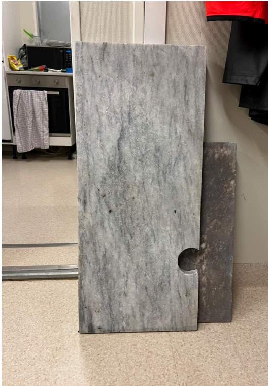
Preservation of the facade requires testing a small sample of panels for structural stability. The test involves boring a hole in the stone which then makes it unsuitable for reuse on the facade.
