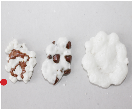
Image 3-8 Filling, Firing bone china with perlite first and filling the gap by red clay and then fired again
