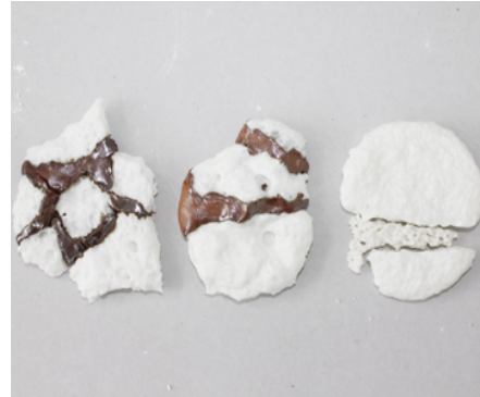
Image 3-7 Comparing the red clay and bone china with mok 2 and bone china with perlite when setting them closely
