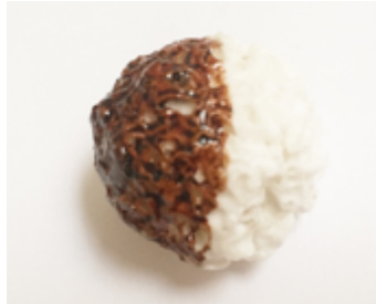
Image 3-15 Dipping bone china with perlite into the lacquer
