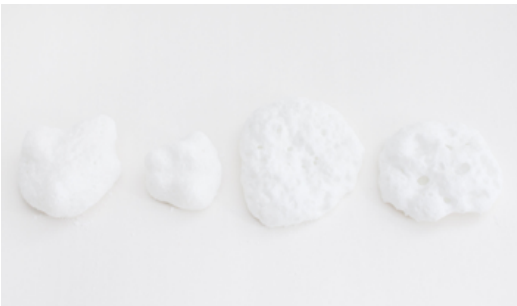
Image 3-2 From the left to right, the frit mok2 are 25%, 35%, 45% and 55% added
