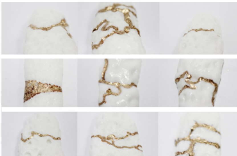
Image 3-14 Creating mending tracks on the bone china with frit mok2 added
