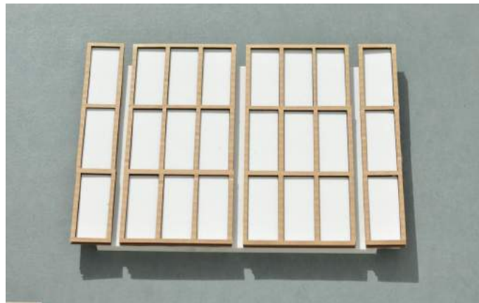
Front panels are fixed to building frame behind, divided using a shadow gap.
