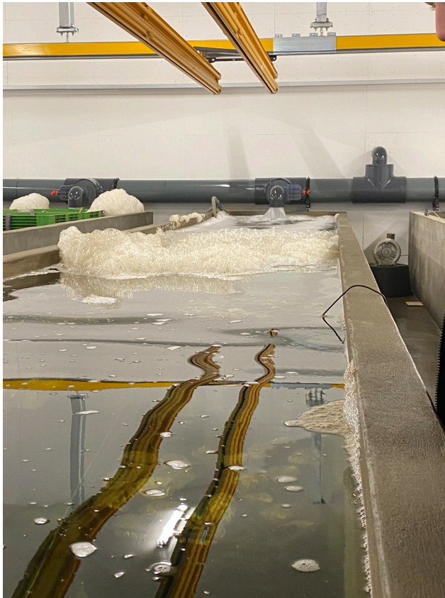
The new basins made espeicailly for oysters are build to fit the plastic trays in which in the oysters are placed for cleaning. For the cleaning process is created a water system ensuring a cirkulation of the water.
